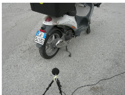
Figure 7: Microphone position during exhaust system noise measurements (stationary two wheel vehicle).
