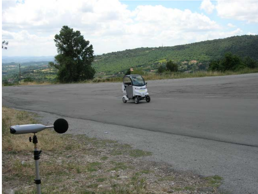
Figure 4: Microphone position during SEL measurements on gradient road (hybrid vehicle in motion).
