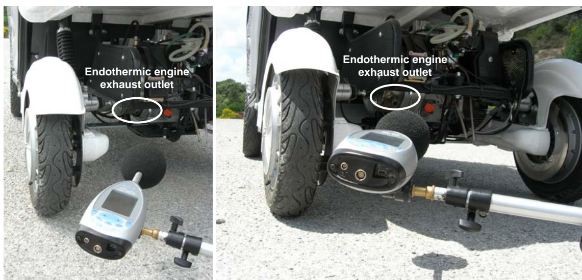
Figure 3: Microphone position during exhaust system noise measurements (stationary hybrid vehicle).
