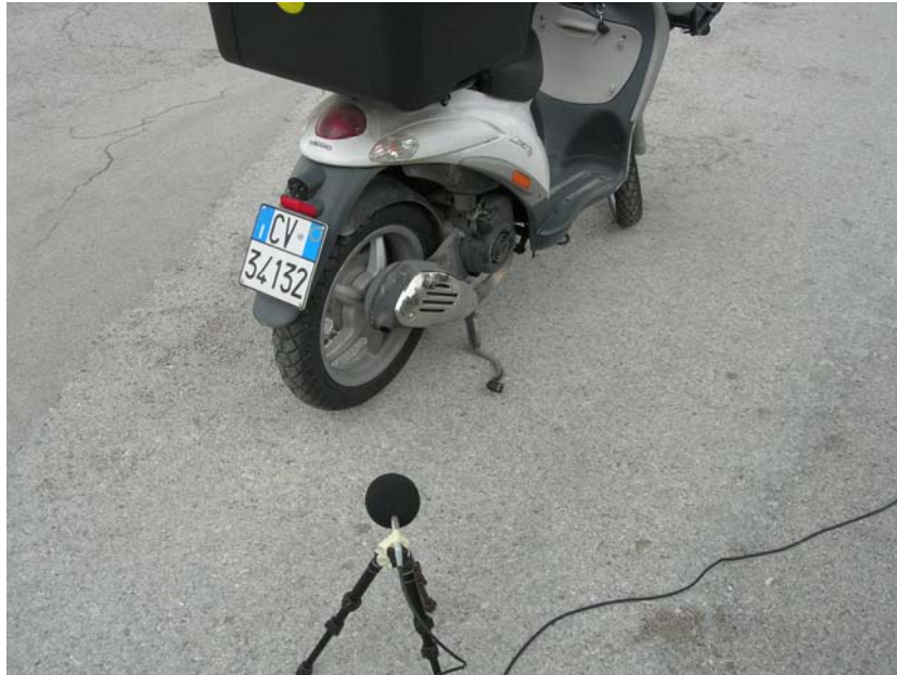
Figure 7: Microphone position during exhaust system noise measurements (stationary two wheel vehicle).
