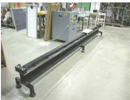
Fig. 16: segment of customized electric linear motor for Pipe§net
